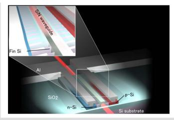
Silicon laser diodes will dramatically increase network speed and reduce power consumption in IT devices. Stimulated emission, a necessary condition to realize the practical application of silicon laser diode, was observed in a device structure suitable for mass production.
